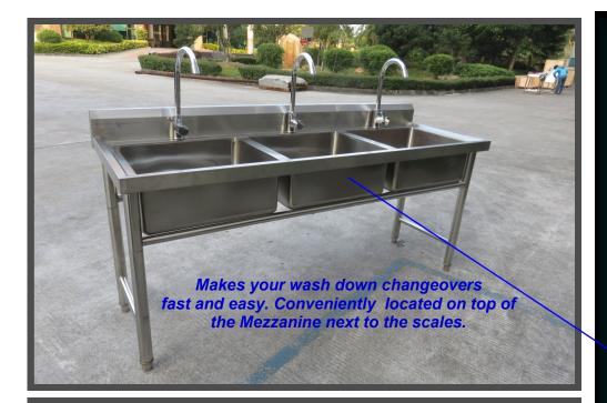
Mounted on top of mezzanine the 3 stage sink eliminates the operators from having to go up and down the stairs of the mezzanine to clean the buckets of the combination scales or other filling equipment.
