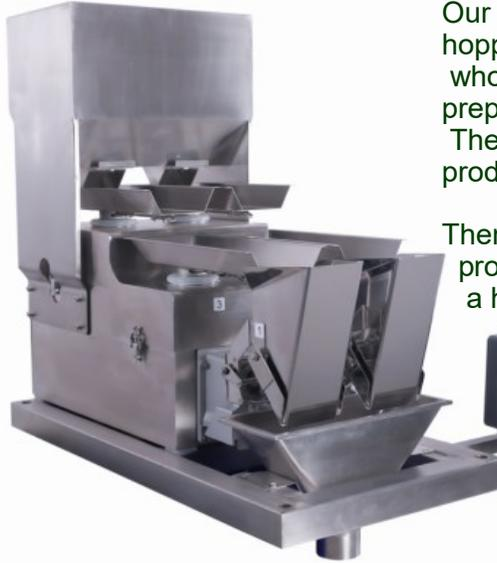
Our nut scale is easy to use: fill the hopper with product, pieces, halves or whole pecans... even spices. Access a preprogrammed target weight. The scale automatically delivers the product to the weigh bucket.
